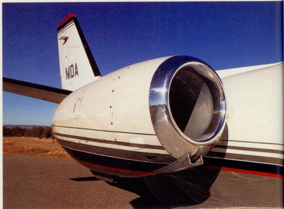
The Sierra Stallion engine mod includes new cowlings to house the Williams International FJ44-2A engines, which weigh less and have a smaller diameter than the original Pratt & Whitney.
